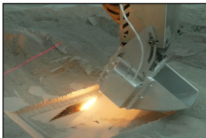
ICON's Prototype Laser VMX toolhead in atmospheric lunar regolith simulant test bed at ICON's Off-Planet Systems lab in Austin, TX.
